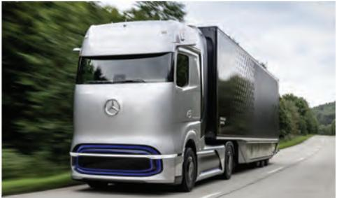
LH2 could double range and capabilities for heavy-duty long-haul trucks (between 1.7 and 2.5 times more than 700 and 350 bar).
