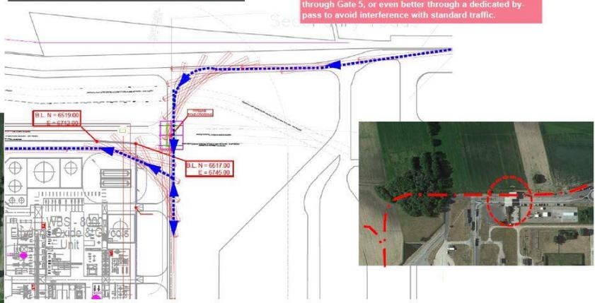
Having studied several solutions, Contractor considers as the most suitable for this oversized equipment the one through Gate 5, or even better through a dedicated bypass to avoid interference with standard traffic.
