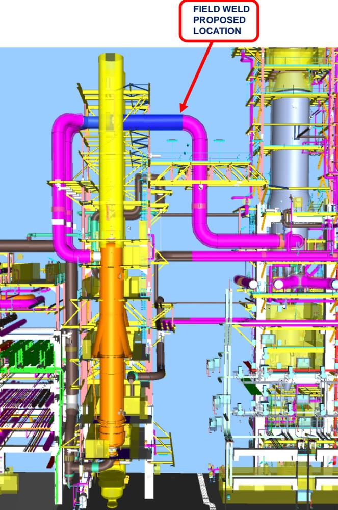
HORIZONTAL SPOOL CONNECTED THE TWO RISERS WILL BE DROPPED CONSIDERING TO LEAVE OPEN THE TOP PORTION OF HCFE STRUCTURE.
