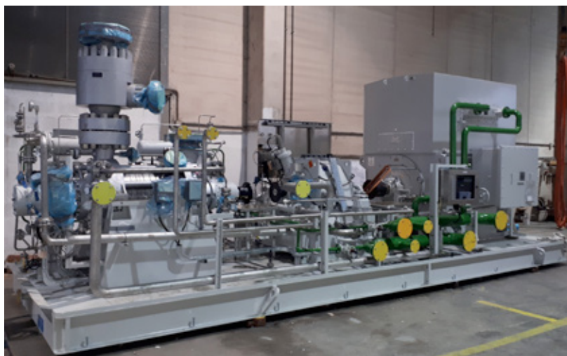
La Pompa DDHF/R a divisione radiale (BB4). ©2024 Baker Hughes Company (All rights reserved)
