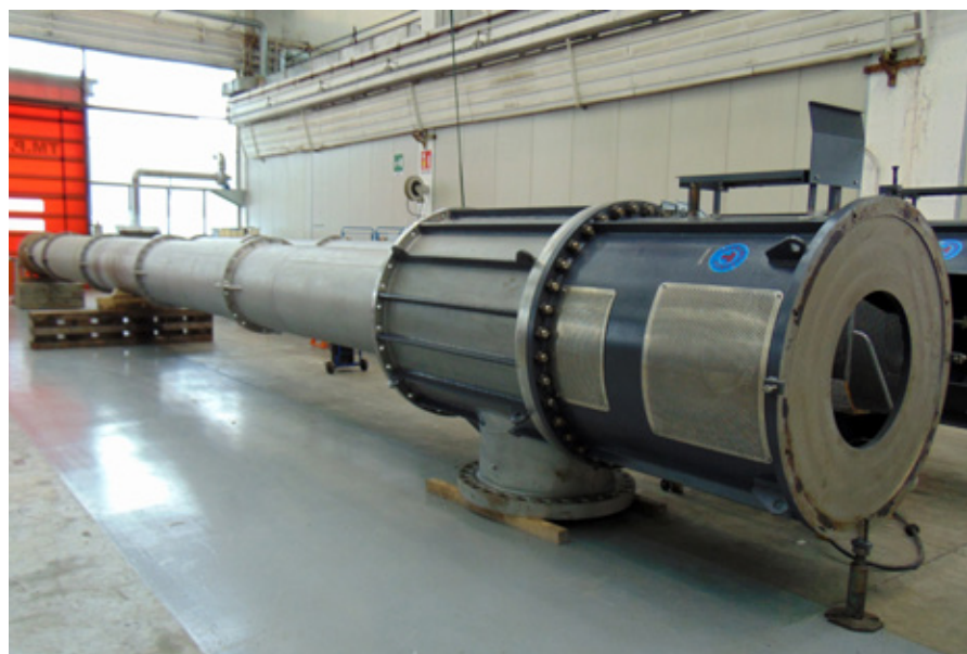
Trillium VS1-type pull out vertical pump for sea water supply at desalination plant
