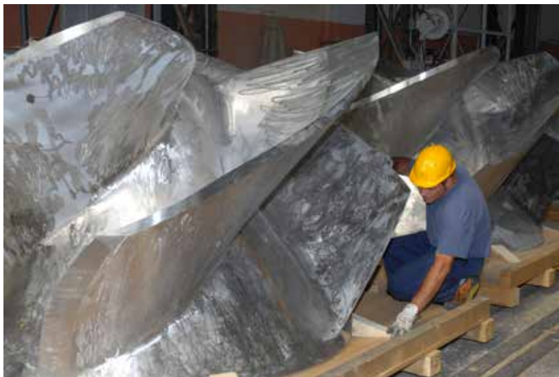
Land Reclamation Project - Concrete volute pump - impeller
