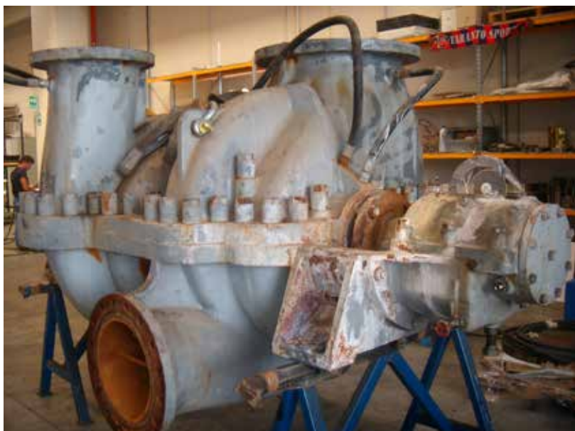
Lifting Station Project - old BB1-type pump design from the 1970s
