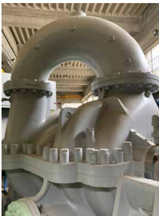
Lifting Station Project - new patented Termomeccanica Pompe HSS between bearing pump design
