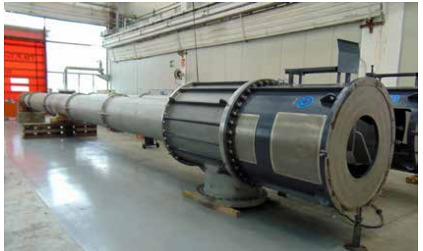
VS1-type pull-out vertical pump for sea water supply at desalination plant
