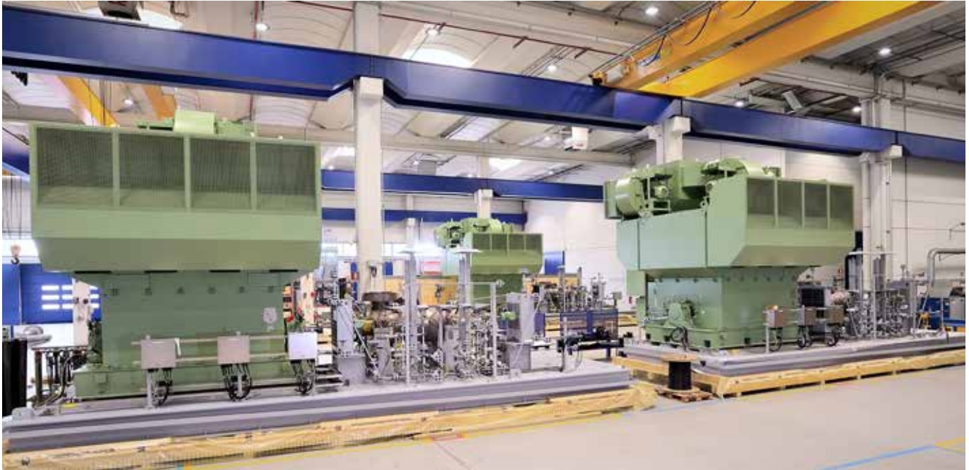
API BB5 type pump for water injection service at oil extraction facility
