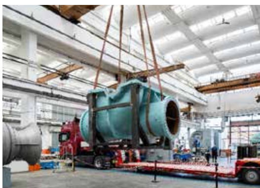
Figure 3 - A Trillium high-capacity split-case pump for cooling water service – Capacity 18,250 m 3 /h – Power 3.3MW
