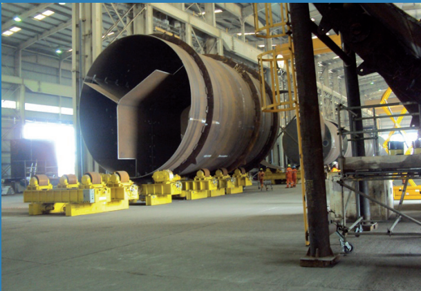
Fig. 9 – Risers anchoring piles at Saipem's yard in Port Harcourt
