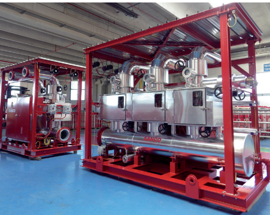
Fig. 3 - Deluge valve units for low temperatures
