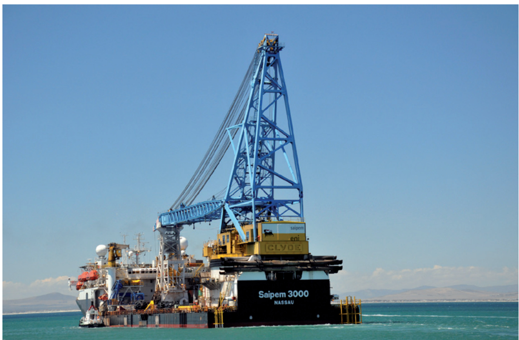
Fig. 4 - Saipem 3000 heavy lift DP vessel
