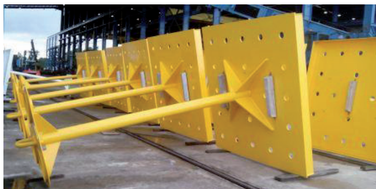
Fig. 7 – Completed LBL array structures at EWT yard in Port Harcourt
