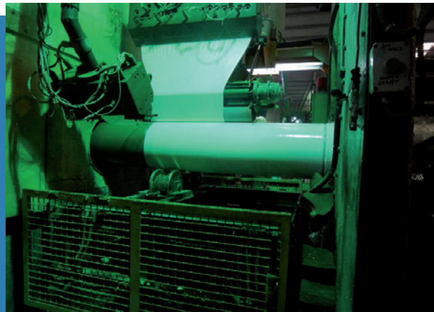
Fig. 11 – Coating of line pipes
