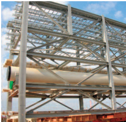
[Figure 7.4 – Pre-dressed Pipe Rack (IREM)]
