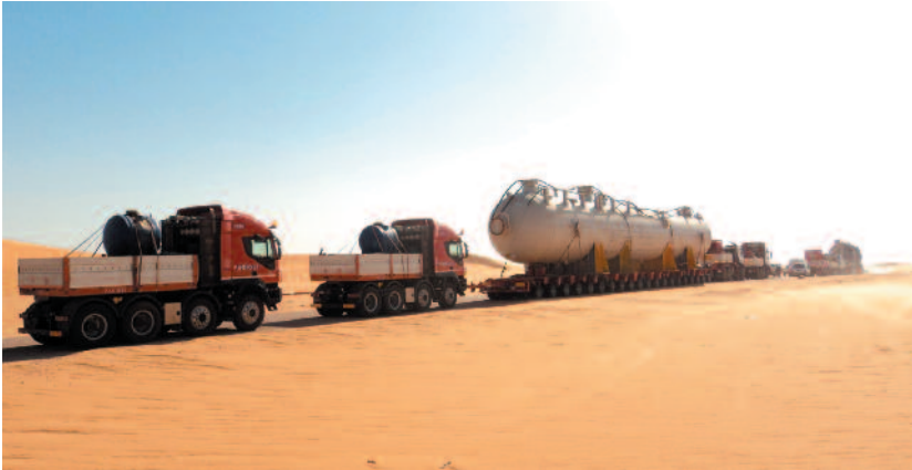
[Figure 12.2 – Vessel transport in Morocco (Fagioli)]
