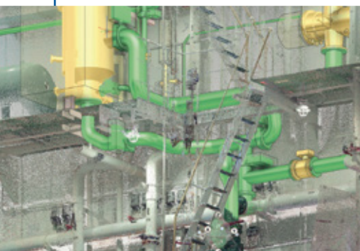
New pipe arrangement for Ballast Water Treatment (Image courtesy of IHB ShipDesign)
