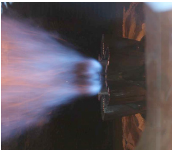
Figure 6 - Mars II – Natural gas flame – Thermal Duty : 35 MWth
