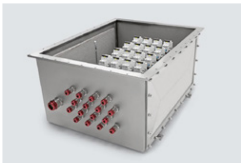
The side walls feature permeable pressure-relief elements, are closed off on the outside by blowout panels and have IP66-rated protection
